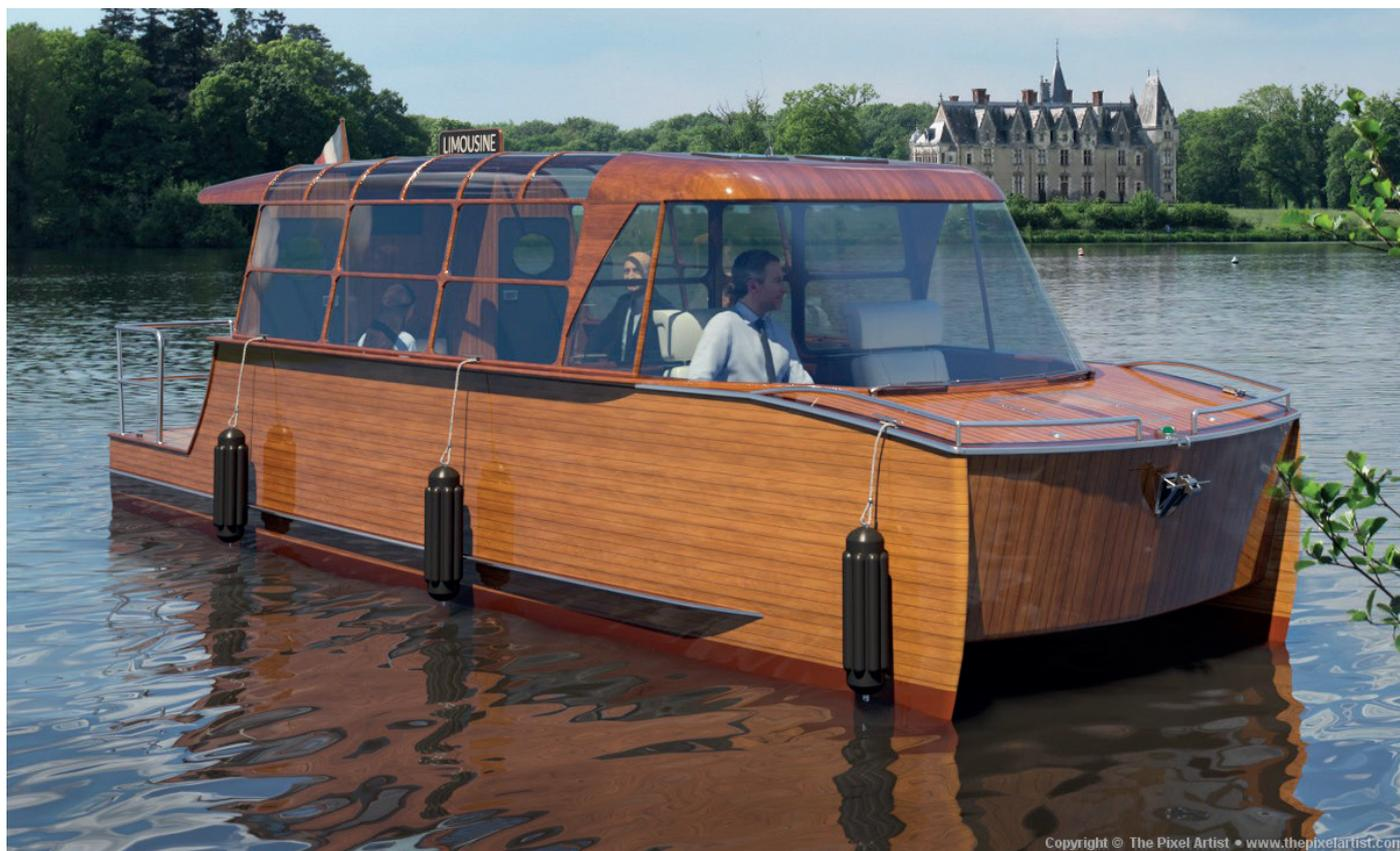
The «**Bateau Limousine**» is a premium mode of transport with chauffeur. The boats wooden construction and large open windows offer a charm unique, combining tradition and modernity. The electric propulsion system with batteries provide a revolutionary water limousine ; silent, ecologic and economic for all your private events or transport for up to 10 passengers.
